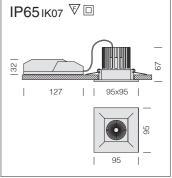
Reflector: screened anti-glare. With lens for better light distribution.
