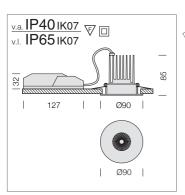
Optics: anti-glare, screened optics. LED: Luminous flux maintenance 70% 50.000h (L70B50).
