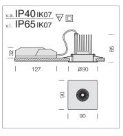
Optics: anti-glare, screened optics. LED: Luminous flux maintenance 70% 50.000h (L70B50).
