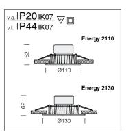
**LED:** Luminous flux maintenance L70B50: 40.000h. Power factor >0.9
