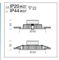
**LED:** Luminous flux maintenance L70B50: 40.000h. Power factor >0.9
